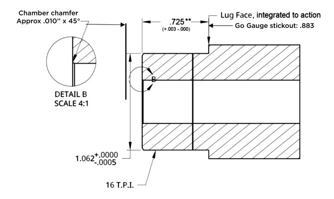
Headspace Tolerance: .885" +/- .001" 0.010" depth with approximately 30° angle is sufficient - user preference.
